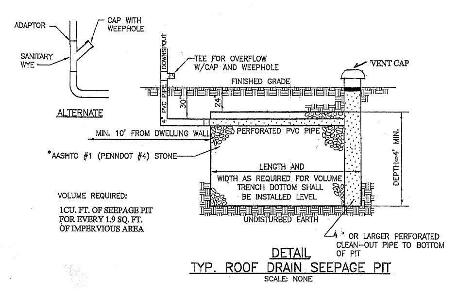
\* TOP 12" OF STONE MAY BE ¼" IN SIZE TO AID IN PIPE INSTALLATION TRENCH SHALL BE LINED WITH PADOT CLASS 1 GEOTEXTILE MATERIAL PER PUBLICATION 408, SECTION 212.36. ALLOW 1' OVERLAP ACROSS BACKFILL AT TOP OF TRENCH AND ALSO AN OVERLAP OF 1' AT END OF ROLLS.
